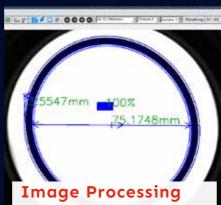
The intuitive image processing software NELA VisionCheck offers the option of creating customised inspection programmes for each specific application.
