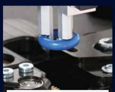
**Indexing Systems** With an individual handling of each part, ROVI provides a significant extension of optical inspection possibilities with tactile inspection, 360° rotation, or crack detection.
