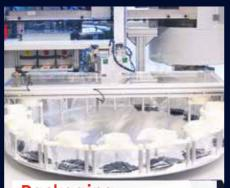
Packaging Gentle sorting of good parts via belt chutes into linear and rotary indexing batchers or bag packers. Integration with existing customer systems possible.
