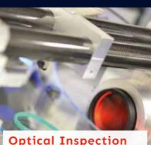
Inspection of surfaces and parting lines as well as dimensions including shape and position tolerances at high throughput rates.
