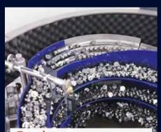
Integration of fully automatic feeding units like bowl feeders, turntables, or handling systems tailored to individual applications. Bunkers
